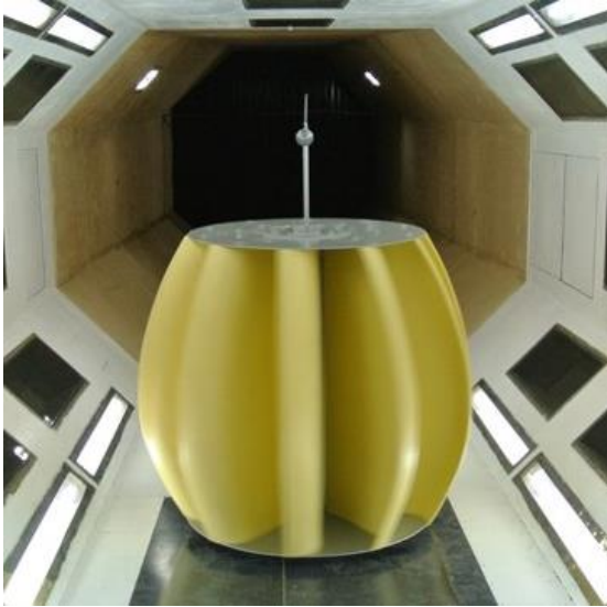
Figure 7. Vertical-axis wind turbine in the wind tunnel and turbine's blade.
